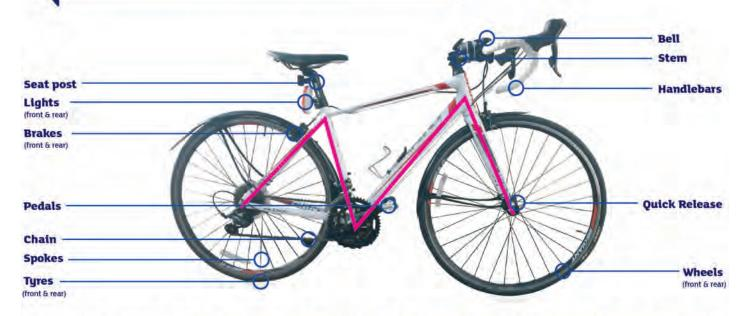
Follow the frame of the bike from the rear wheel up to the saddle, down to the pedals, up to the handlebars and down to the front wheel. This is your **M-check**.
