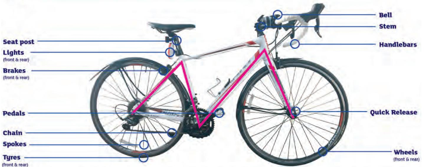
Follow the frame of the bike from the rear wheel up to the saddle, down to the pedals, up to the handlebars and down to the front wheel. This is your **M-check**.
